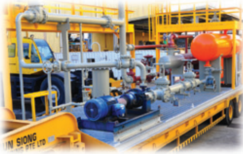
Fabrication and Assembly of Skid
