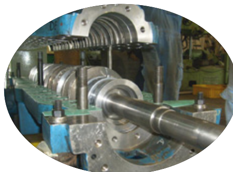
Multistage pump overhauling
